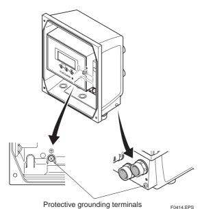
Figure 4.4.4 Protective Grounding Terminal Location
